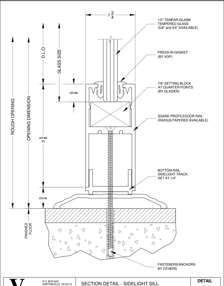
PHONE: 800-368-3011 276-956-3020 SECTION DETAIL - SIDELIGHT SILL 3-5/8" SQUARE RAIL w/ 1/2" THRESHOLD 24
